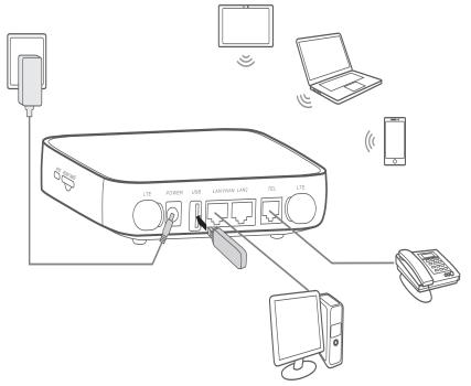
To prevent interference caused by radio signals, place the Cat7 Router at least one metre away from phones and other electrical devices.
